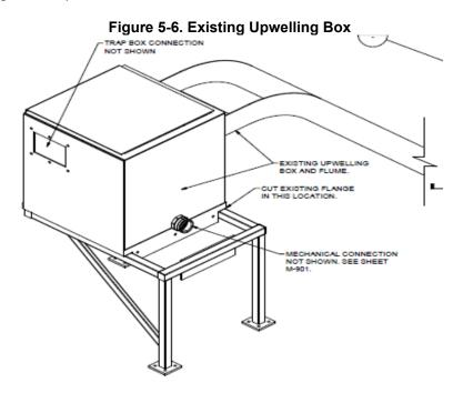
A new manifold will connect the LPS supply piping to the upwelling box. The manifold will use two control valves. One valve will control flow into the upwelling box. A portion of the remaining flow will be diverted into the new trap box as supplemental supply water. This allows the system to eliminate heat transferred from the environment into the trap box (see Figure 5-7).
