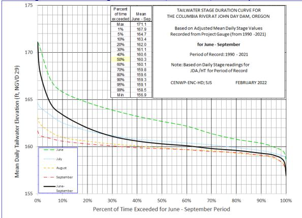
Figure 3-5. Tailwater Stage Duration Curve; 1990 to 2021; June to September.
