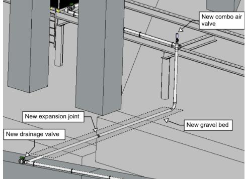
Figure 5-4. LPS Supply Piping at Platform
