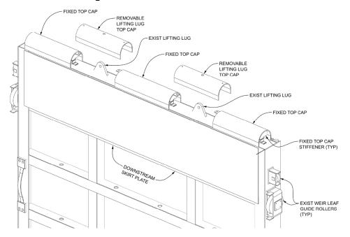
Figure 4-3. Downstream Side of Weir
