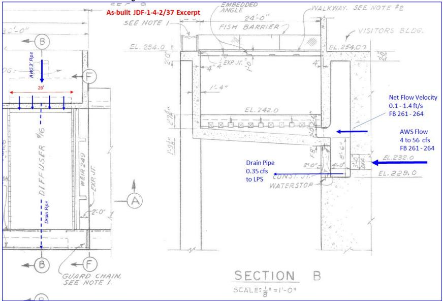
Figure 3-8. As-built Plan and Elevation Views of Diffuser 16.
