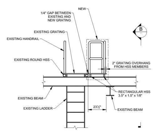
The handrail on the existing platform will be shifted to the outside edge of the new platform. Project staff will need to order a new 22.5-inch long handrail for the portion of
