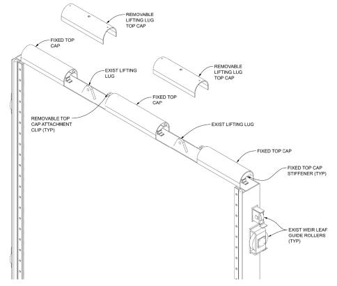
Figure 4-2. Upstream Side of Weir showing Rounded Top Cap Mod
