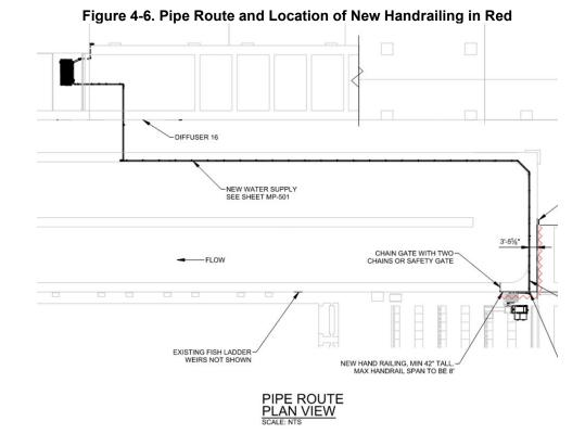
Figure 4-6 shows the pipe route and location of handrailing.
