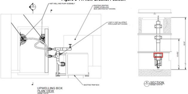
Figure 5-11. New Bracket Position
